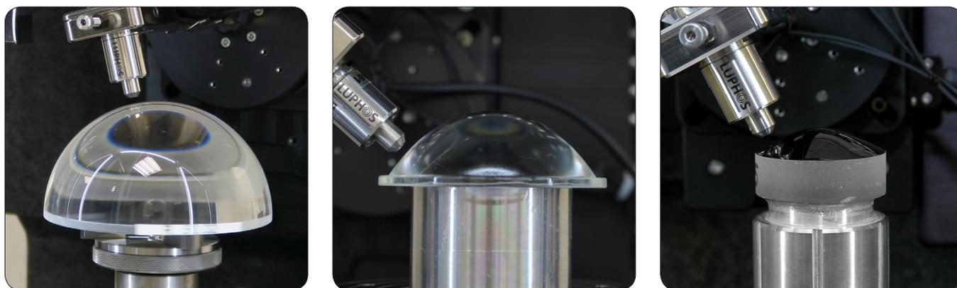
LuphoScan platforms are scanning interferometers based on an optical (non-contact) point probe that utilizes MWLI<sup>®</sup> technology (multi-wavelength interferometry).
